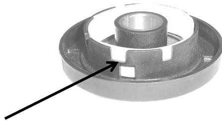
The thin area between the crank position and the cylinder position is the most common breakout location.
