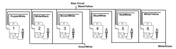
12. Replace the CDM Modules one at a time until the defective CDM Module(s) are identified.
