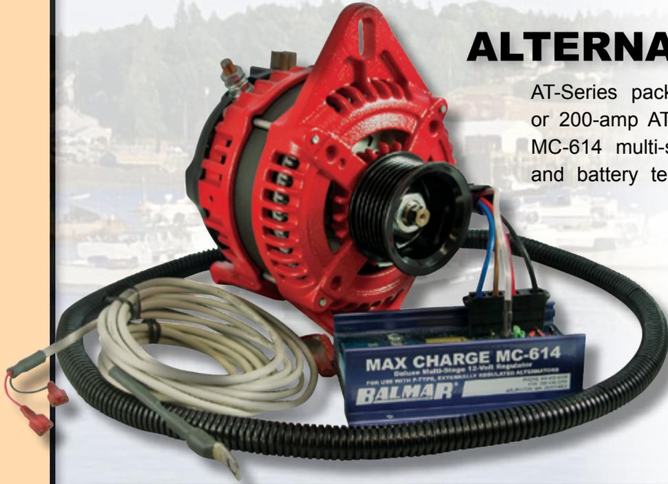
AT-Series packages combine high output 165-amp or 200-amp AT-Series alternators with our intelligent MC-614 multi-stage regulator, along with alternator and battery temperature sensors, to deliver a pre-matched system that's ready to take on the tough charging challenges. Packages are available in single-foot, or dual-foot saddle style mounting configurations.
